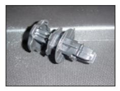
**S T E P** 6 There are two anchors for cargo in the upper corners of the rear plastic trim panel. These two anchors need to be removed in order to remove the trim panel. To remove these, pull on the outside of the anchor top section it will pull out, allowing the anchor itself to collapse and be pulled out.
